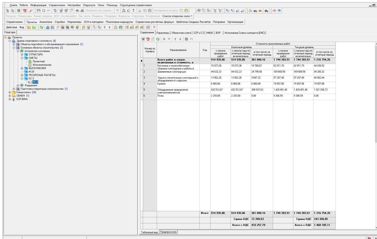
The screenshot shows the Smeta.RU software interface with the 'КС-3' report open. On the left, there is a tree view of project structures under 'Проекты'. On the right, a large table displays the breakdown of work and costs by item, showing values for both base and current prices.
